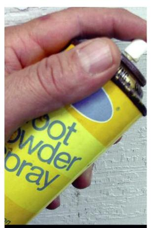
An old trick is to clean the engine, spray likely areas with aerosol foot powder, then watch for oil tracks.
