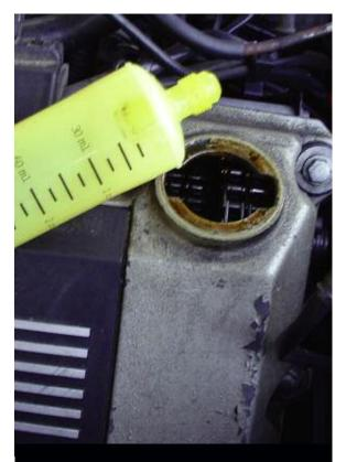
Just an ounce of dye will do the trick no matter how much oil the crankcase contains.
